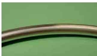
Figure 2: Parker Hannifin's Silver-Indium diffused plating
